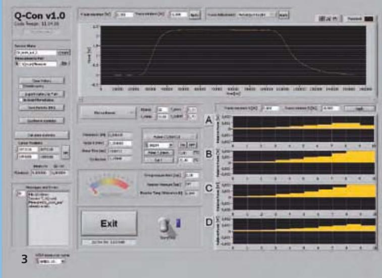
The modular design of “concal” makes it possible to adapt the sensor arrays to different microreactors with differing dimensions and applications. A selection of processes that have already been analysed using “concal” shows the broad applicability of the measurement system for the calorimetric characterisation of chemical reactions in microreactors:
